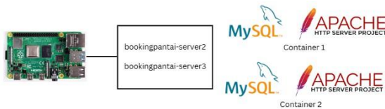
Fig 5 Beach Booking App Deployment Architecture on Raspberry Pi
