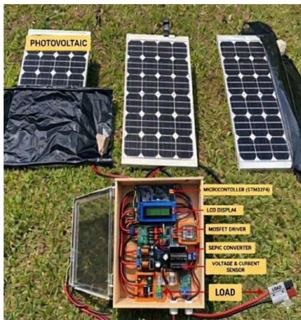
Fig. 7. Experimental prototype of the photovoltaic MPPT system.
