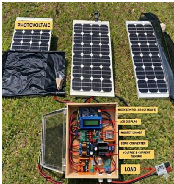
Fig. 7. Experimental prototype of the photovoltaic MPPT system.
