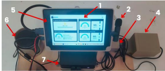
Description: 1. Navienta Application 2. JETE Mic Bluetooth 3. TTL / CAN to USB converter for TF LiDAR 4. TF350 Ultra Long Range Single-point LiDAR 5. LCD 7 Inch HDMI 1024x600 6. Bluetooth Speaker 7. Intel NUC 13 Pro (NUC13ANH7)
