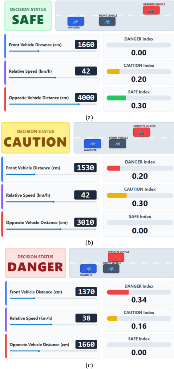
Fig. 5. Simulation-based validation showing the fuzzy logic decision spectrum: (a) Safe status at 1660 cm gap, (b) Caution status at 3010 cm gap, and (c) Danger status at 1660 cm gap with high relative velocity.
