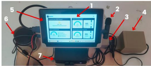
Description: 1. Navienta Application 2. JETE Mic Bluetooth 3. TTL / CAN to USB converter for TF LIDAR 4. TF350 Ultra Long Range Single-point LIDAR 5. LCD 7 Inch HDMI 1024x600 6. Bluetooth Speaker 7. Intel NUC 13 Pro (NUC13ANHi7)
