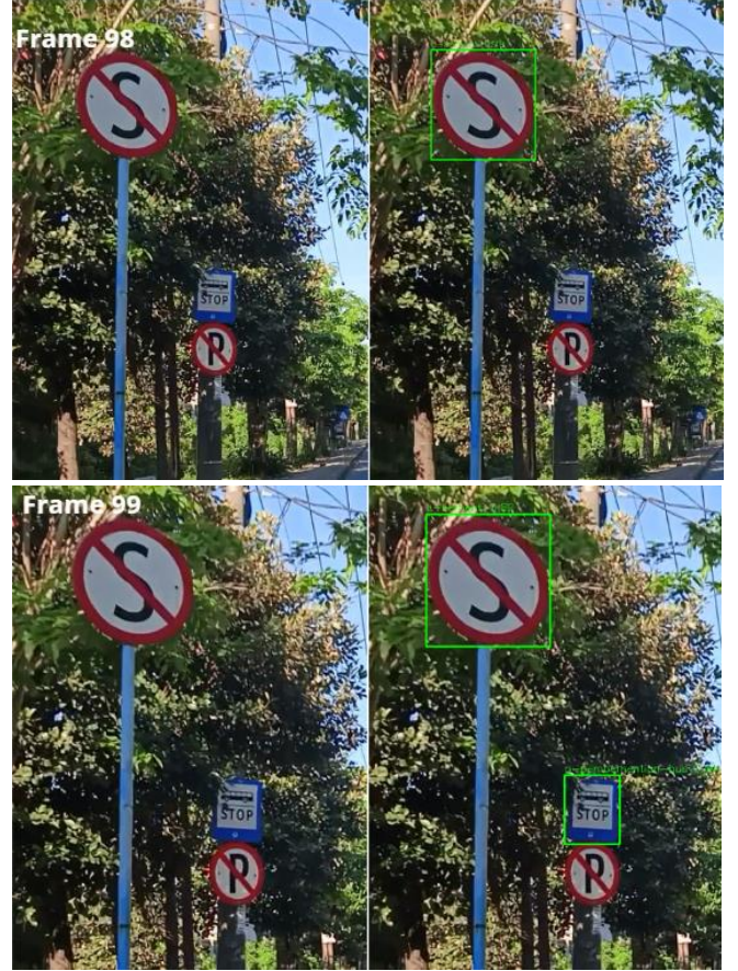
Fig. 6. Example of false detection suppression using motion-consistent filtering.
