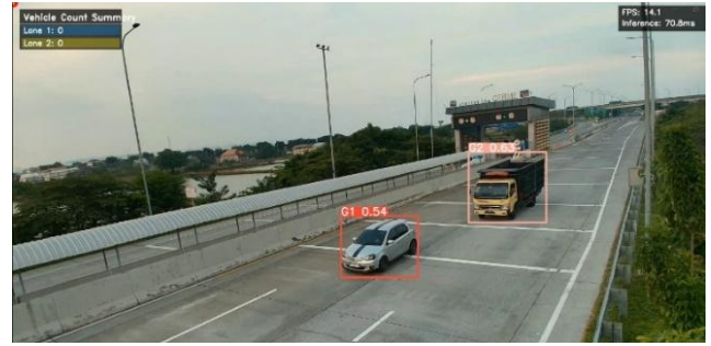
Fig 7. Result detection and classification in multi-lane and vehicle
