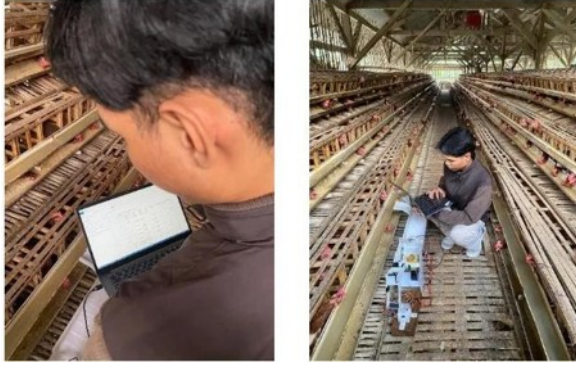
Fig. 4. Data collection at the laying-hen farm in Desa Biting, Arjasa, Jember. Left: operator monitoring real-time grading on laptop. Right: SORTA hardware deployed between egg cages during testing
